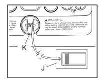
displays will light. IMPORTANT: In an emergency, the key can be pulled from the console, causing the walking belt to slow to a stop. Test the clip by carefully taking a few steps backward; if the key is not pulled from the console, adjust the position of the clip.
