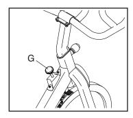
To stop the flywheel, push the resistance knob downward. The flywheel should quickly come to a complete stop.
