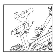
firmly tighten the adjustment knob. Make sure that the adjustment knob is engaged in an adjustment hole.
