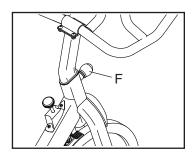
hole in the handlebar post, and firmly tighten the adjustment knob. Make sure that the adjustment knob is engaged in an adjustment hole.
