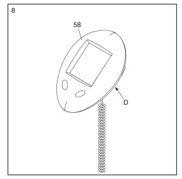
9. Slide the Console (58) onto the Console Bracket (10) on the Handlebar (7).
