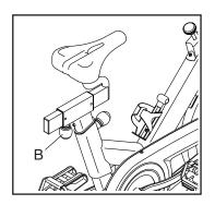
tighten the adjustment knob. Make sure that the adjustment knob is engaged in an adjustment hole.
