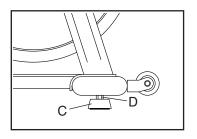
each leveling foot, loosen the leveling foot and the nut (D) above it, adjust the leveling foot to the desired position, and then tighten the nut against the stabilizer.
