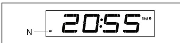
**To manually advance the scan cycle**, press the Scan button repeatedly.
