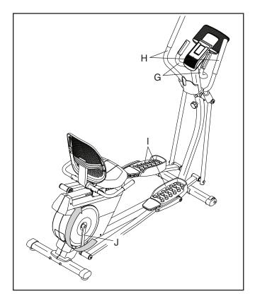
Push the pedals (I) until they begin to move with a continuous motion. Note: The crank arms (J) can turn in either direction. It is recommended that you move the crank arms in the direction shown by the arrow; however, for variety, you can turn the crank arms in the opposite direction.
