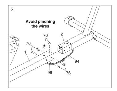
Locate the wire tie (E) in the top of the Upright (2), and pull the Upper Wire (94) out of the Upright. Then, untie and discard the wire tie.
