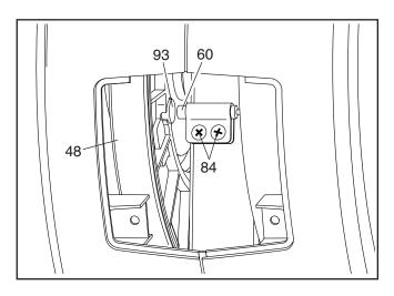
Next, rotate the Large Pulley (48) until a Pulley Magnet (93) is aligned with the Reed Switch (60). Slide the Reed Switch slightly toward or away from the Pulley Magnet. Then, retighten the M4 x 16mm Screws (84).
