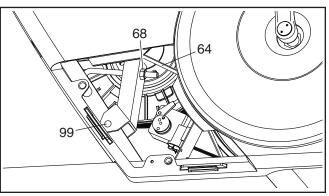
When the Drive Belt (64) is tight, tighten the M10 x 55mm Shoulder Bolt (99). Then, reattach the side access cover.
