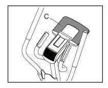
To insert a tablet or smart phone into the tablet holder (C), set the bottom edge of the tablet or smart phone in the tray. **Make sure that the tablet or smart phone is firmly secured in the tablet holder.** Reverse these actions to remove the tablet or smart phone from the tablet holder.
