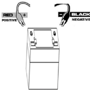
REMOVE TIMER KIT COVER AND INSTALL A 6V RECHARGEABLE BATTERY (NOT INCLUDED) BY ATTACHING RED ALLIGATOR CLIP TO THE POSITIVE (+) AND BLACK ALLIGATOR CLIP TO THE NEGATIVE (-) TERMINAL.
