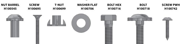
To help with assembly we recommend sorting your hardware bags with the seven digit alpha-numeric number printed on the bags or by hardware type (i.e. bolts, nuts, etc.). Organizing your hardware will make assembly easier.
