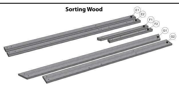
When removing the wood from the boxes we recommend arranging them by part number before you begin assembly. This will allow for faster assembly and easily identify any parts that may be missing or damaged.
