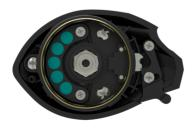
MAGNETIC BRAKE ADJUSTMENT: After you set the spool tension, you can reset the magnetic brake dial to your preferred setting. With dual brakes, you also need the magnetic dial on zero to set tension. Dual brake reels work best if you set the internal pins to control the cast for most conditions and then set the magnetic dial to compensate for wind or late fluff up during a cast.
