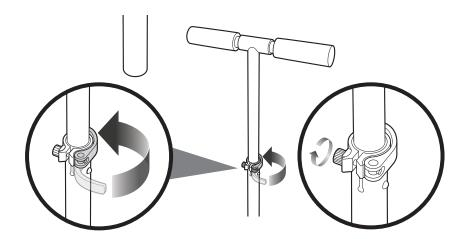
**2** The tension of the quick-release lever can be adjusted by manually tightening or loosening the Allen bolt. Be careful not to over-tighten. You should always be able to open and close the quick-release lever by hand and the T-bar should slide freely when the quick-release lever is open.
