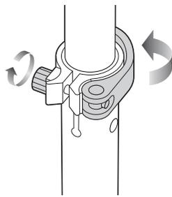
**1** To adjust the height of the handlebars, open the quick-release lever and slide the T-bar to the desired position and resecure the quick-release lever to lock into place. When the T-bar is raised to the maximum height, depress the push button located directly below the quick-release lever to unlock the T-bar.
