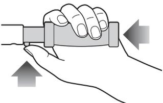
**2** Insert and secure the left and right handlebars by pressing the spring-loaded buttons and inserting them into the T-bar.
