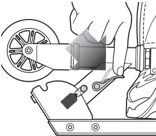
**1** To release the folding mechanism, place the scooter on the ground, put one foot on the deck plate and push joint release lever down. Raise T-bar up until it is securely locked in the upright position.
