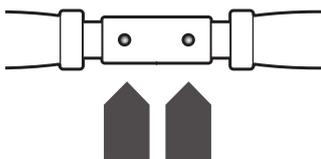
**3** Make certain **BOTH** handlebars are properly locked onto the T-bar.
