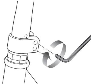
**2** With the front wheel pointed straight ahead and the handlebars square to the front wheel and the Razor logo facing the front, tighten the clamp as shown. Tighten securely. On the A4, alternately tighten each bolt until securely tightened.
