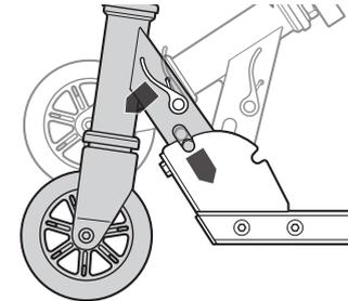
**Note:** The joint release lever is spring-loaded and will automatically lock in the upright position when fully upright.
