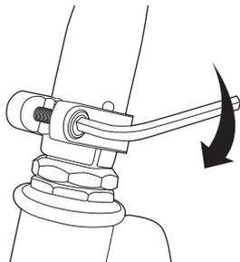
Using a 5 mm Allen wrench, check that the collar clamp bolt(s) are tightened securely. This item is tightened and quality inspected at the factory, but there is a slight chance that the effects of shipping or handling may have caused the bolt(s) to loosen.
