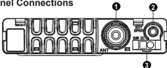
1. **ANT Jack** - SO-239 UHF connector for external antenna (included)
