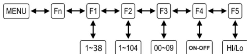
**F1- CTCSS Codes.** Use this option to select and assign a Continuous Tone Coded Squelch System (CTCSS) Privacy Code for the currently active channel.
