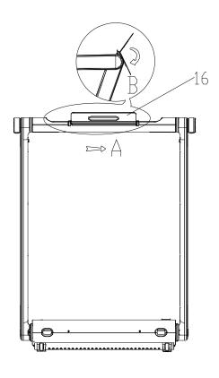
Before folding the treadmill, stand in front of the treadmill. Fold the **Pad Bracket (No. 16)** upward by pulling it to the right as shown in drawing A. Then, turn it down as shown in drawing B.
