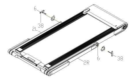
Tighten 2 Nuts (No. 6) to Left & Right Upright (No. 2L & No. 2R) using the Tool (No. 38).
