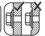
**Note:** Pre-drill all holes using a 1/8" drill bit before installing the Pan Screws.
