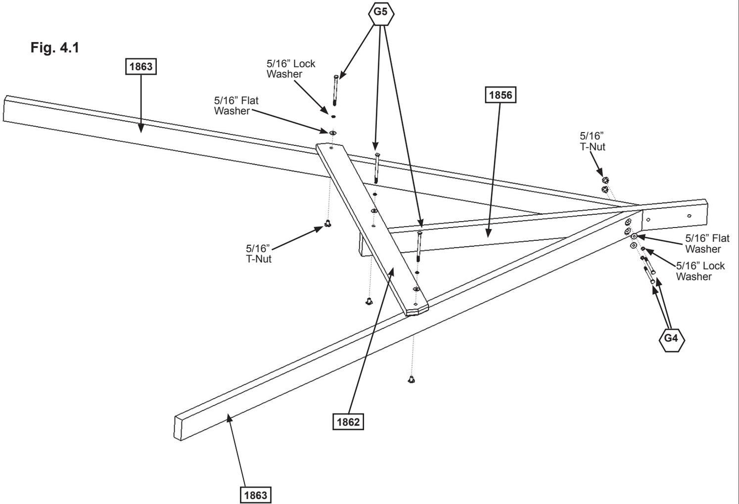
**B:** Attach (1862) SW Support to both (1863) SW Posts and (1856) SW Upright using 3 (G5) 5/16 x 4-1/2" Hex Bolts (with lock washer, flat washer and t-nut). (fig. 4.1)
