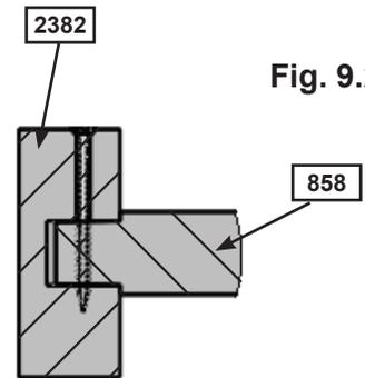
**B:** Make sure shoulder of dowel is against each post before pre-drilling pilot holes. Drill 1/8" pilot holes through the posts and into the dowel to prevent splitting. (fig. 9.2 and 9.3)
