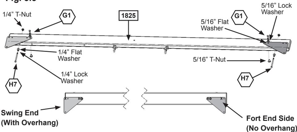
**D:** Attach 1 (H7) 1/4 x 5-1/2" Hex Bolt (with lock washer, flat washer and t-nut) to the ends of each (1826) Front Beam and (1825) Back Beam. The bolts do not attach to anything, but **MUST** be installed to the beams to prevent splitting and checking of wood. (fig. 3.2 and 3.3)
