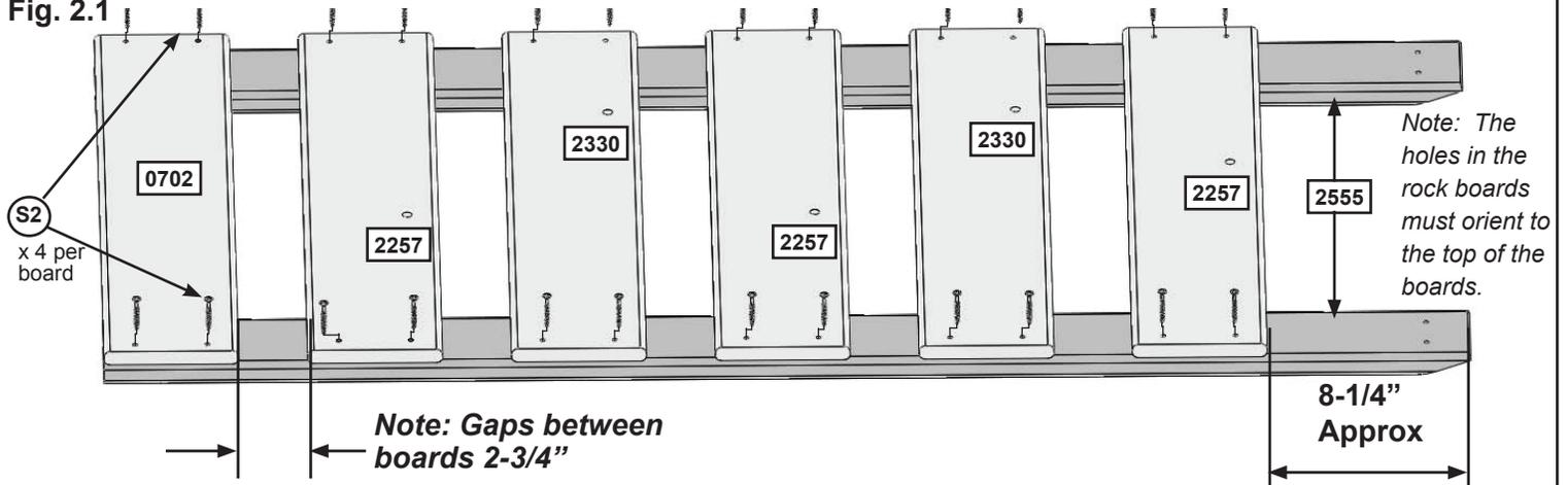
**A:** Lay 2 (2555) Rock Rails down, side by side with angled edges facing down. (fig. 2.1)
