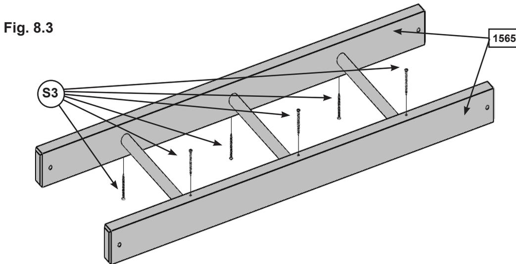
**C:** Attach (578) 1-1/8 x 15-7/8" Dowels to both rails with 2 (S3) #8 x 2-1/2" Wood Screws per dowel. (fig. 8.3)
