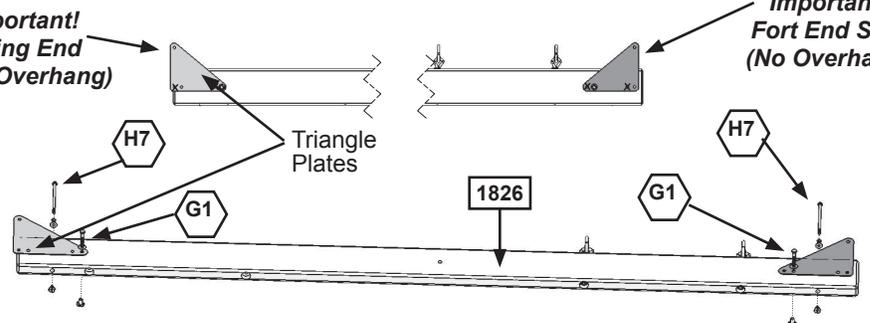
**C:** Attach 1 Triangle Plate to the ends of each (1826) Front Beam and (1825) Back Beam using 1 (G1) 5/16 x 1-1/2" Hex Bolt (with lock washer, flat washer and t-nut) per triangle plate in the hole indicated in fig. 3.2 and 3.3. **Correct hole usage is very important.**
