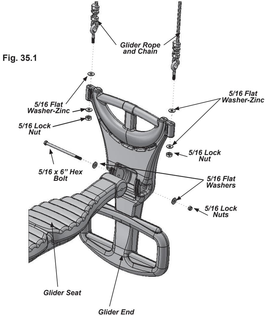
**⚠ WARNING:** Bolt must not exceed 1/2 thread past the nut
