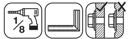
**Note: Pre-drill all holes using a 1/8" drill bit before installing the Lag Screws.**
