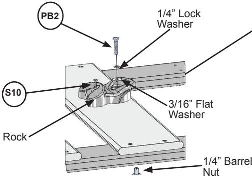
**E:** Place 1 rock on each rock board (fig. 2.2) and attach using 1 (PB2) 1/4 x 1-1/4" Pan Bolt (with lock washer, flat washer and barrel nut) and 1 (S10) #8 x 1" Pan Screw per rock. The Screw must be in the hole directly under the Pan Bolt, it will stop the rock from spinning. (fig. 2.3)
