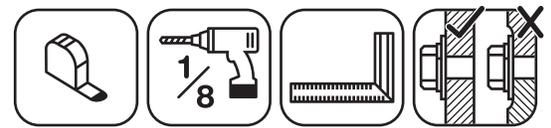
**Note: Pre-drill all holes using a 1/8" drill bit before installing the Lag Screws.**
