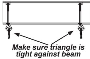
**WARNING:** For your child's safety, orientate the swing hangers as shown to ensure your swing will have proper swing motion when installed. Failure to do so could result in premature failure of the swing hanger or swing chain.
