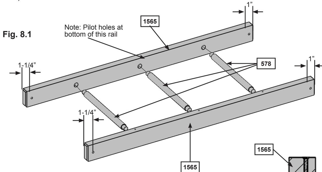
**B:** Make sure shoulder of dowel is against each rail before pre-drilling pilot holes. Drill 1/8" pilot holes through the rails and into the dowels to prevent splitting. (fig. 8.2)
