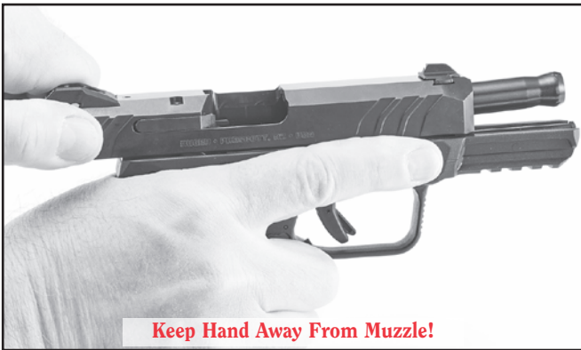
Figure 4 Retracting the Slide
