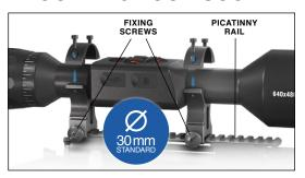
The ThOR 4 has a 3.5-inch eye relief, and can be mounted using 30 mm mounting rings. ATN has provided two standard rings and one L shape ring. The L shape ring is for those instances when you need extra eye relief for certain rifles. First, choose your preference of rings and position and mount the bottom portions of your rings to your rail for optimal eye
