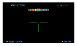
Movement between the colors is carried out using the LEFT and RIGHT buttons . Press the OK button to accept your color.
