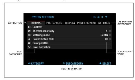
On the left side of the Tab Bar you will find the Exit (with arrow icon). Selecting Exit and pressing the OK button will bring you back to the Homescreen. Movement between the tabs is carried out using the LEFT and RIGHT buttons
