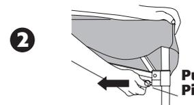
Release pull pin at each corner by first lifting fabric away from slider. With one hand push up on truss near the pull pin, pull the pin out to release.
