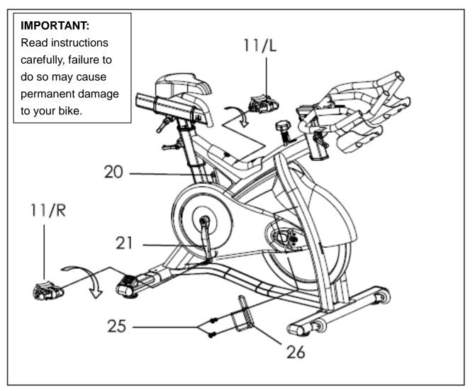
Connect **Pedals L/R (11)** onto the **Left** and **Right Crank Arm (20 and 21)**. (Before you begin, immobilize the crank arms by turning the tension control knob all the way to the right).
