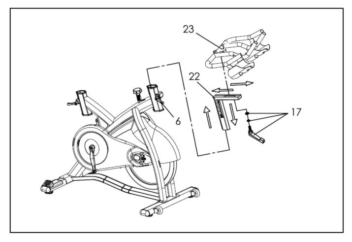
Insert the **Handlebar Post (22)** into the head tube of the Main Frame. Move **Handlebar Post (22)** to the desired height. Tighten the **Release Lever (6)** to secure the **Handlebar Post (22)** into position.
