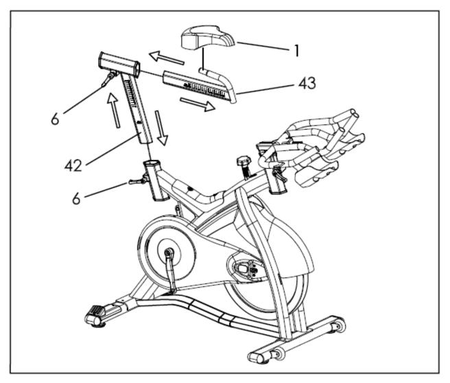
Insert the Seat Post (42) into the seat tube located on the Main Frame.
