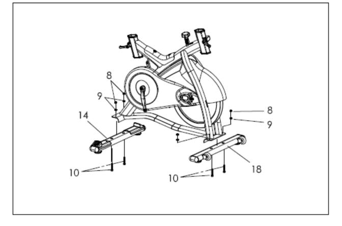
Attach the **Front Stabilizer (18)** and the **Rear Stabilizer (14)** to the Main Frame using 4 **Bolts (10)**, 4 **Washers (9)** and 4 **Nuts (8)**. Tighten and secure using spanner wrench.
