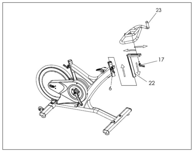
Insert the **Handlebar Post (22)** into the head tube of the Main Frame. Move **Handlebar Post (22)** to the desired height. Tighten the **Release lever (6)** to secure the **Handlebar Post (22)** into position.
