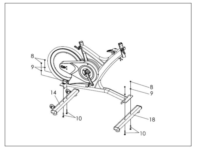
Attach the **Front Stabilizer (18)** and the **Rear Stabilizer (14)** to the Main Frame using 4 **Bolts (10)**, 4 **Washers (9)** and 4 **Nuts (8)**. Tighten and secure using spanner wrench.
