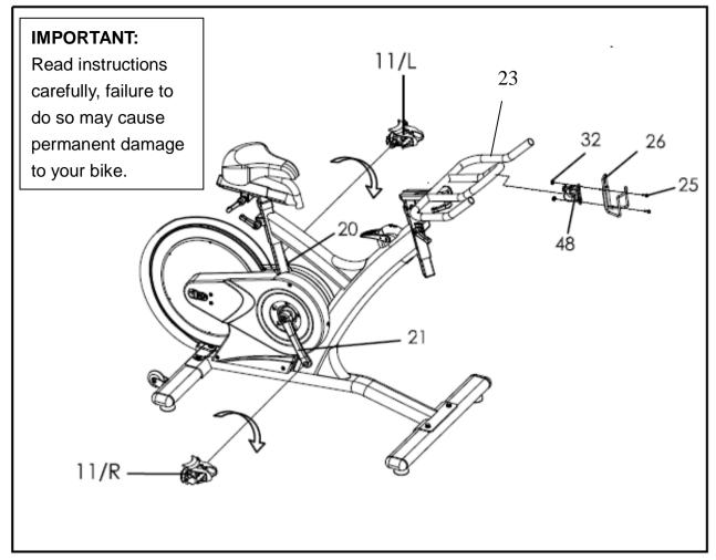
Connect **Pedals L/R (11)** onto the **Left** and **Right Crank Arms (20 and 21)**. (Before you begin, immobilize the crank arms by turning the tension control adjuster all the way to the right).
