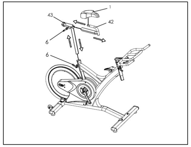
Insert the Seat Post (43) into the seat tube located on the Main Frame.
