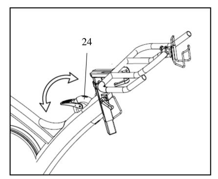
Adjust the exercise resistance on the bike using the **Tension Adjuster (24)** to increase (-) or decrease (+) resistance.
