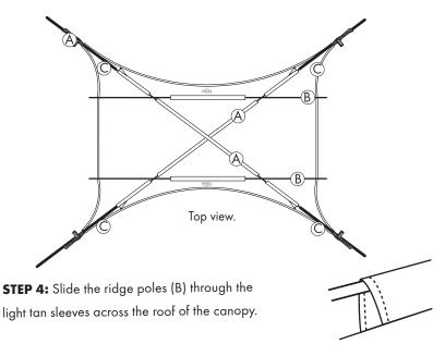
**STEP 5:** Extend the four steel poles (C), by pulling out each wire-corded section and placing the jointed ends into the connected pole sections.
