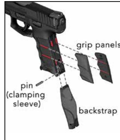
Figure 5 Installing backstrap and grip panels
