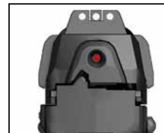
Figure 11 — Firing pin cocked
