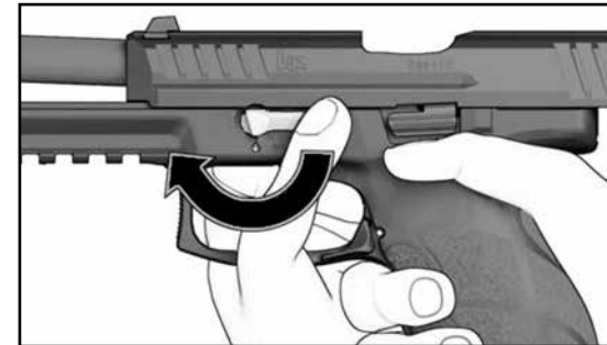
Figure 14 — Rotating the disassembly lever
