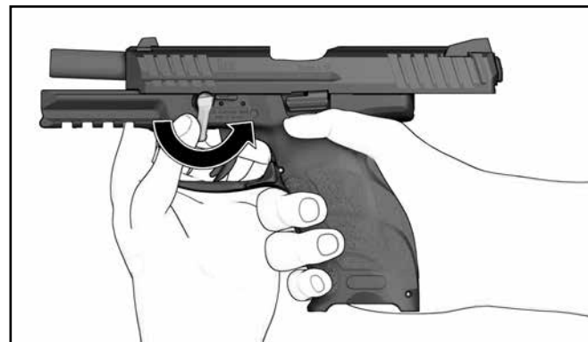
Figure 28 — Pivot the disassembly lever counter clockwise
