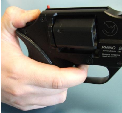
Figure 3: Releasing the external hammer
