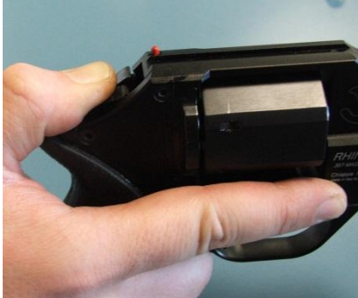
Figure 1 : Cocking the external hammer
