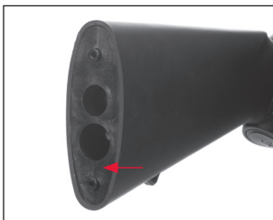
Remove the stock insert.
