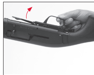
Lift the trigger group from the receiver.
