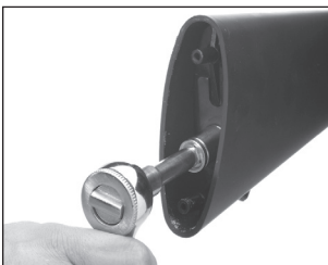
Use a socket wrench to remove the stock bolt.
