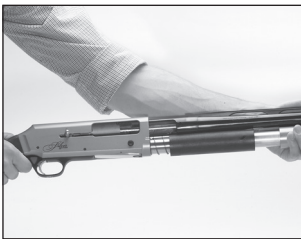
Slide the barrel and piston over the magazine tube and the barrel extension into the receiver.
