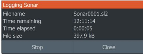
→ **Note:** If you have selected the Create StructureMap option in the record sonar dialog, the Convert structure log to map dialog is displayed when you select Stop in the Logging Sonar dialog. Select Convert to create a smf file in the Log folder. Refer to "Files" on page 78.
