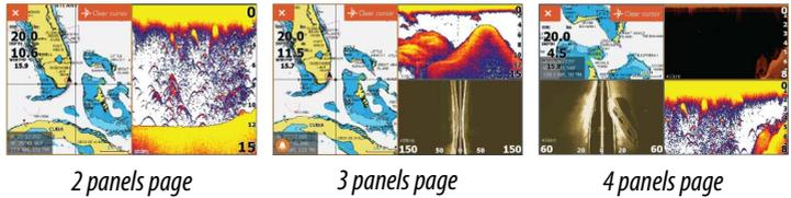
Panel sizes in a multiple panel page can be adjusted from the System Controls dialog. Refer to "Adjusting the split on multiple panel pages" on page 21.
