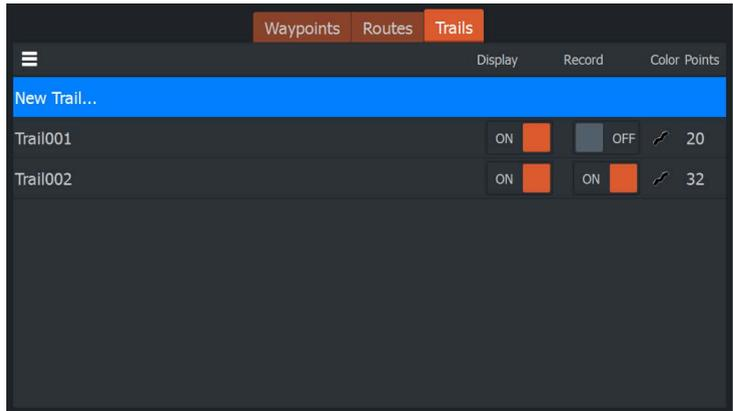
From the factory, the system is set to automatically track and draw the vessel's movement on the panel. The system continues to record the trail until the length reaches the maximum points, and then automatically begins overwriting the oldest points.
