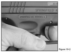
Striker Block Safety - As an added safety feature, an internal striker block will prevent the firearm from firing until the grip safety is depressed and the trigger is pulled.
