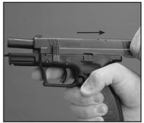
7. Move the complete slide assembly forward and off the frame (See Figure 27-2.)
