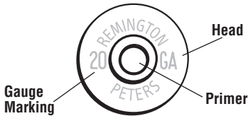
PICTURE 2 This picture shows the parts of the ammunition.
