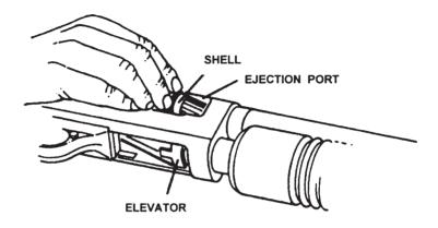
Fig. 5 -- Loading through the ejection port
