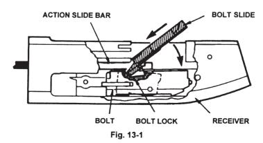
Hold the bolt slide down and pull the forearm assembly forward. The bolt and bolt slide should move freely in their cuts in the receiver. If parts do not slide easily – **DO NOT FORCE** – disassemble and reassemble, paying attention to the relationship of the bolt, bolt slide and action slide bars.
