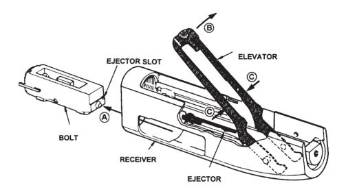
Fig. 11 -- Elevator removal
