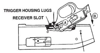
TRIGGER HOUSING PIN HOLE
