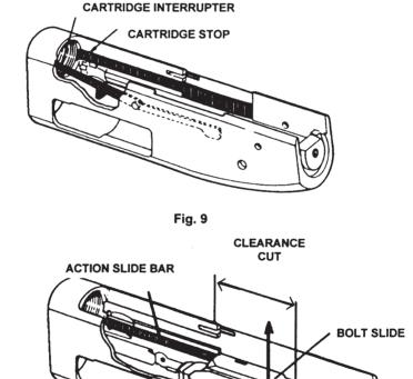
Fig. 10 - Bolt slide installation/removal
