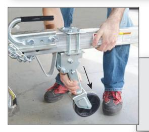
Tip: To improve performance, apply 2-3 drops of SAE 30 engine oil to each side of the wheel and pivot assembly at least semi-annually.
