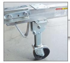
Place the Top Mounting Plate over the tongue and aligned with the bottom mounting plate.
