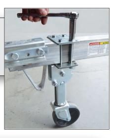
To place in the transport position, lift up on the trailer tongue while pulling down on the spring loaded leg.
