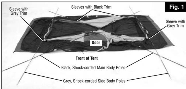
4. Insert end of each black Main Body Poles & grey Side Body Poles into pins. (Fig. 2 & 2A)
