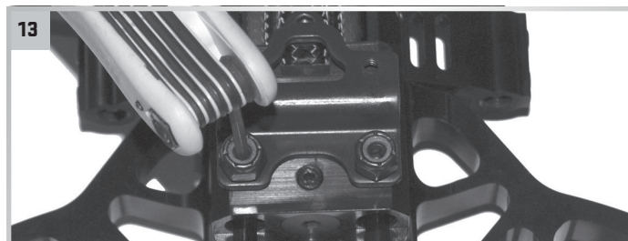
Insert the 3/4-inch setscrews & Nylock nuts (use the 1-inch setscrews for Wicked Ridge crossbows).
