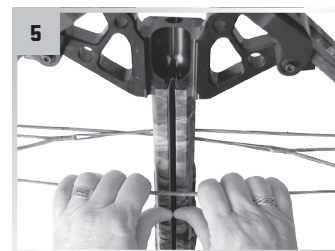
Pull up and back slightly on the bowstring to seat the bow assembly.
