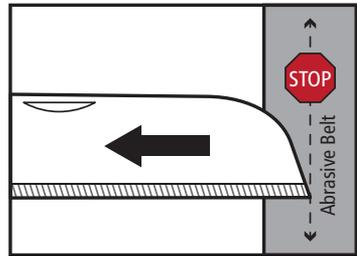
Pull straight through the guide and stop on the middle of the belt. Do not lift the blade handle. Turn power off as knife tip contacts belt.
