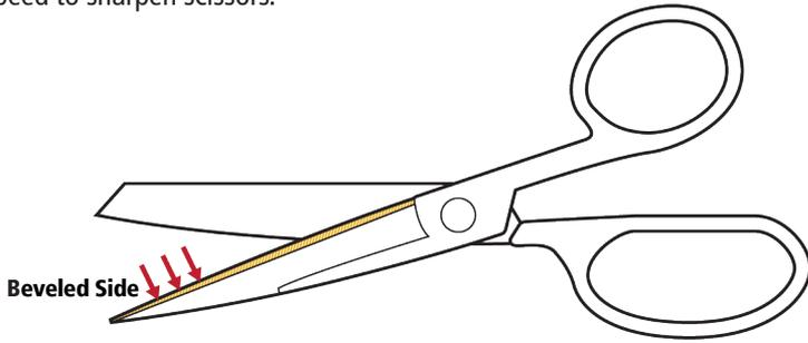
Once scissor blade is properly placed in Sharpening Guide, squeeze power switch and simultaneously pull the scissor blade steadily through the guide.
