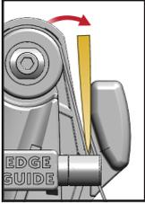
**With power off**, insert blade into right side of sharpening guide all the way to the start of the edge.
