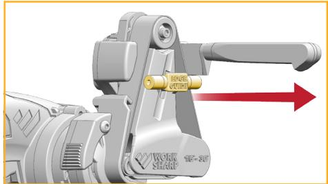
Continue sharpening on right side of guide only until a burr is created along the entire length of the edge or you have reached the recommended stroke count in section 4.
