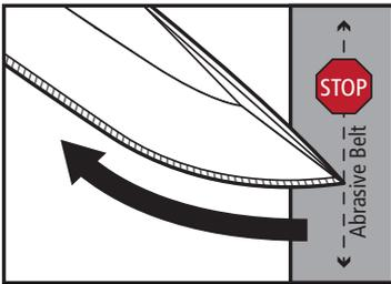
Follow the curve of the blade so the edge remains perpendicular to the belt. Stop on belt.
