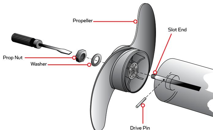
1. Disconnect the motor from all sources of power prior to changing the propeller.
