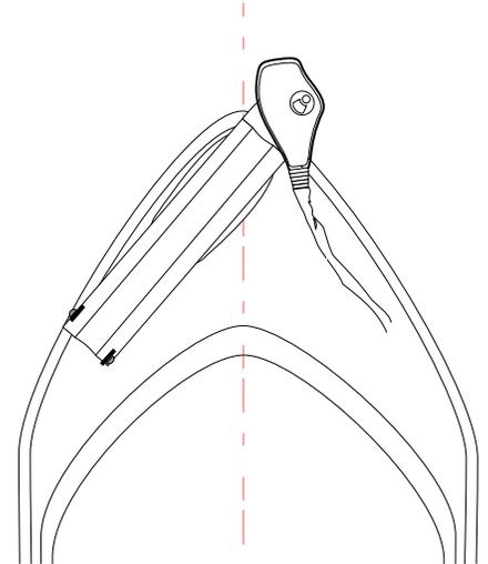
**NOTE:** If pattern 2 is to be used, the right side plate must be removed to access the mounting holes in the bow plate.
