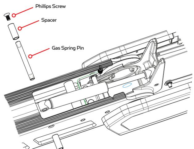
**WARNING: Moving parts can crush or cut. Gas assist lift mechanism is under pressure. Disconnect gas spring before removing motor from mount. Do not pull rope until gas spring is disconnected.**
