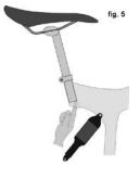
WARNING: A IF YOUR SEAT POST IS NOT INSERTED IN THE SEAT TUBE AS DESCRIBED IN B.1 ABOVE, THE SEAT POST MAY BREAK, WHICH COULD CAUSE YOU TO LOSE CONTROL AND FALL.
