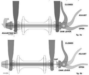
A hollow axle with a shaft ("skewer") running through it which has a nut on one end and a fitting
