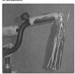
Insert plug end of streamers into grip as shown in the photo above.
