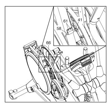
Slightly loosen the two indicated M4 x 16mm Screws (61). Slide the Reed Switch (58) slightly toward or away from the Magnet (41), and then retighten the Screws.
