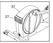
M4 x 16mm Screws (not shown) from the Top Shield (37), and use a standard screwdriver to pry the Top Shield upward off the elliptical.
