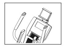
secured in the tablet holder. Rotate the tablet holder to the desired angle. Reverse these actions to remove the tablet from the tablet holder.
