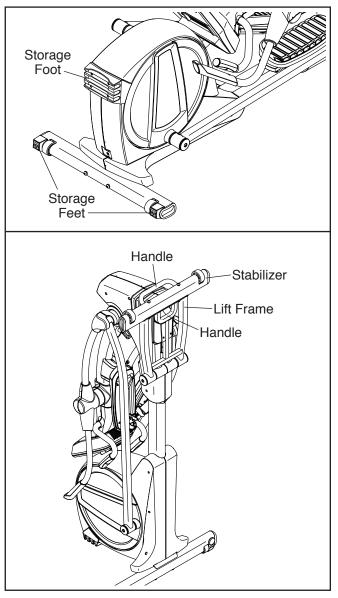
To lower the elliptical for use, first hold the handle on the lift frame with one hand and hold the front stabilizer with your other hand. Next, pull the frame towards you and lower it until you can reach the handle on the front stabilizer. Then, hold the handle on the front stabilizer with both hands and finish lowering the elliptical to the floor.
