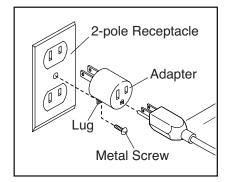
The lug or wire extending from the adapter must be connected with a metal screw to a permanent ground such as a properly grounded outlet box cover. **Some 2-pole receptacle outlet box covers are not grounded. Before using an adapter, contact a qualified electrician to determine whether the outlet box cover is grounded before using an adapter. The temporary adapter should be used only until a properly grounded outlet can be installed by a qualified electrician.**
