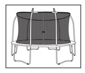
2) Lay Down the entire Net together with the Rods to the Trampoline Mat.
