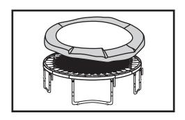
**Step 2:** The pad has double tie strings with an S shaped hook at the end. Attach one S shape hook to the springs of the mat, and the other S shape hook to the V-rings of the mat. Attach the hooks from underneath the mat.
