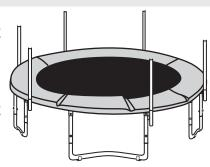
2) Once the lower pole is attached to the part F2, insert the push button on the opposite end of the lower pole, the button should pop out of the hole. You can then attach the upper pole to the lower pole. Continue this step to all the poles. Make sure the foam are covering the poles. Place the pole caps © on top of the poles.
