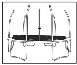
3) Remove all the Poles from Bottom and lay it down to the trampoline.
