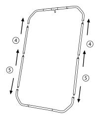
Step 4: With (10) slot facing forward, slide (10) onto (9). Line up (9) hole with (10) slot. Attach (8) with push pin to (9) hole. Push pin will end up in (10) slot.
