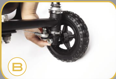
B. Insert Wheel and Attach Nut
