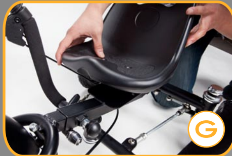
G. Place Screws in Seat on Frame
