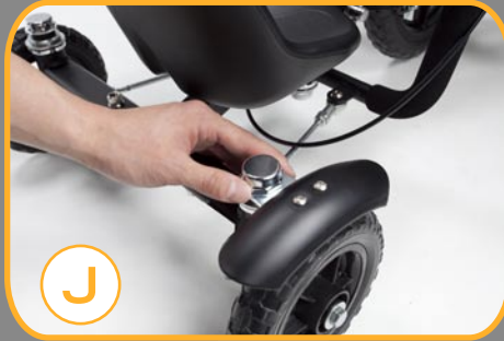
J. Place Fender and Replace Cap
