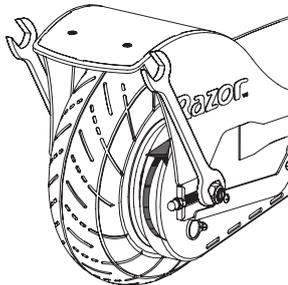
**4** Once the tension is correct, tighten the axle bolts and brake housing anchor bolt. Test ride the scooter. Readjust as needed.
