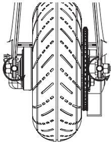
**4** With a 10mm wrench, loosen both axle adjusters an equal amount, approximately five turns.
