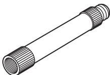
**1** Use the valve extender located inside the end of the right handlebar grip.
