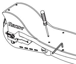
**2** Unscrew the four screws on the middle of the deck with the 4mm key wrench and the Phillips screwdriver.
