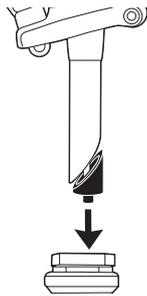
**2** Remove the plastic protector covering the base of the handlebar assembly. Insert the "quill" part of the handlebar assembly into the fork. You may have to loosen the wedge to allow it to slip into the fork.
