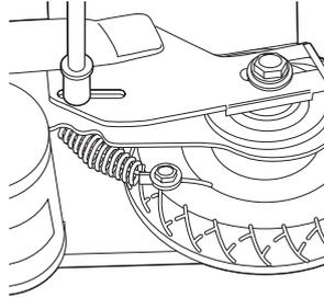
**2** Using two 8mm wrenches, loosen the brake housing anchor bolt which is located in the long slot on the left side of the rear fork.
