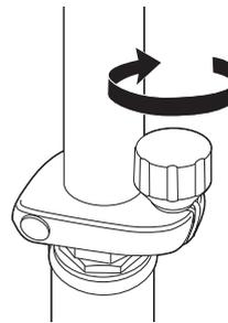
**6** Swing the locking knob to the 12 o'clock position and tighten by hand as firmly as possible.
