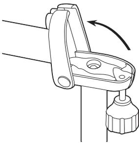
**1** Loosen the locking knob and swing to the 6 o'clock position to unfold the handlebar.
