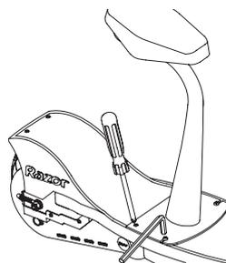
**3** Place the seat post on the deck and secure using the same 4 screws.
