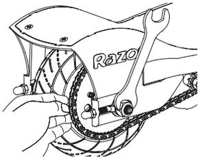
**7** Install new chain or wheel by maneuvering the chain onto the sprocket and slipping the axle into the slots on the frame.
