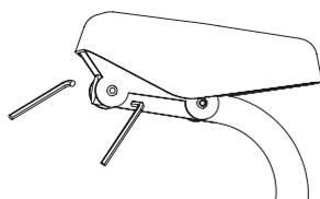
**1** Attach the seat to the seat post with two 4mm key wrenches.
