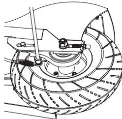
**2** With a 10mm wrench, loosen the brake cable anchor and disconnect the cable.
