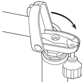
**5** Pivot the handlebar assembly upright.
