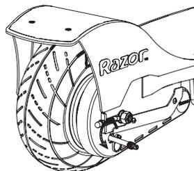
**2** Open the round cover located on the chain cover by sliding the cover upward. Align the opening in the drive sprocket with the valve stem. Thread the adapter completely onto the valve stem and attach the pump. Inflate to the PSI indicated on the tire sidewall.
