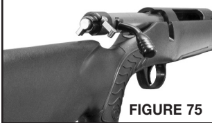
Rotate Bolt Handle Up Until the Bolt Stop Engages the Tracking Groove
