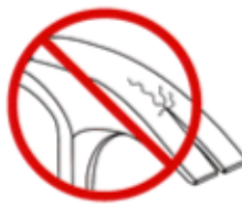
Crack in claw section
