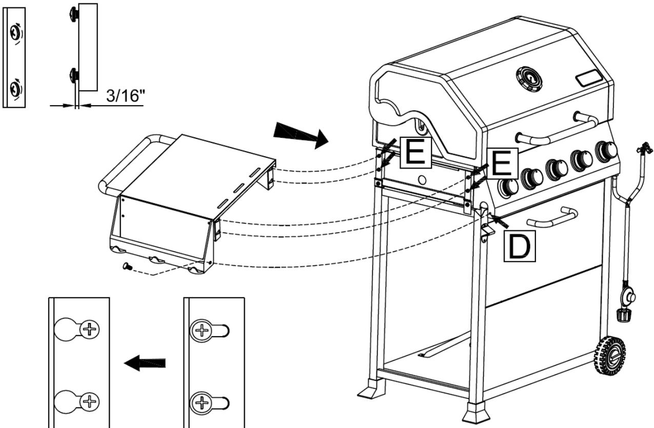
**Step 15:** Attach the **Side Burner Panel Assembly (11)** to **Side Burner Assembly (10)** by using 3 pcs **M6x10 bolts (D)**.
