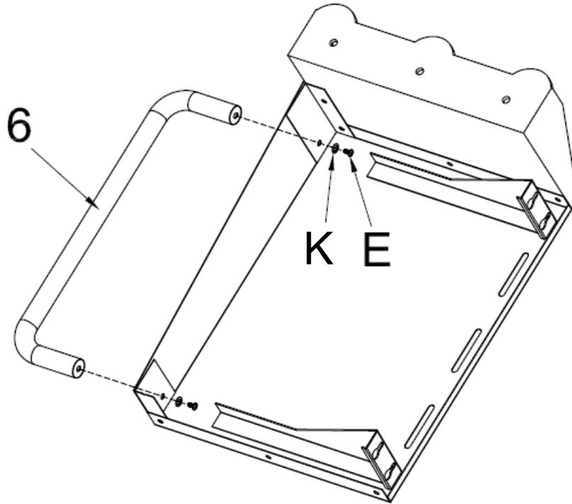
**Step 14:** Remove 1 pc **M6x10mm bolt (D)** at the left side of the control panel. Loosen 4 pcs pre-attached bolts **M6x12 bolts (E)** on left side of the grill body and adjust to 3/16" clearance as shown. Position the holes on the left side table assembly through the bolts at grill body as shown below. Push the left side table leftwards to lock it in place and tighten the bolts **M6x10mm (D)** and **M6x12 bolts (E)**.
