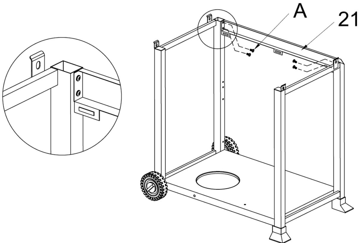
**Step 5.** Attach the **Front Cart Lower Panel (23)** to the cart assembly by using 4 pcs **M5x10 bolts (A)**.
