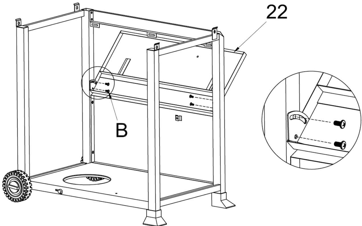
**Step 7.** Attach the **Front Cart Panel Handle (24)** to the front cart upper panel by using 2 pcs **M5x12 bolts (B)**.
