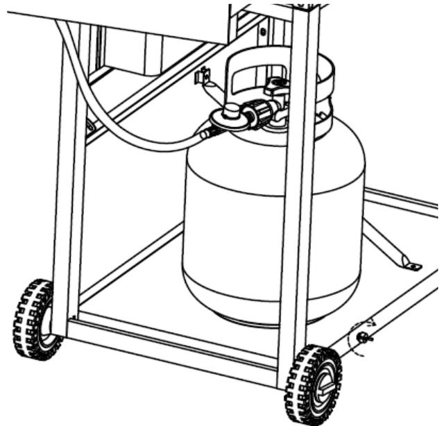
**WARNING: Keep the fuel supply hose away from any heated surfaces.**
