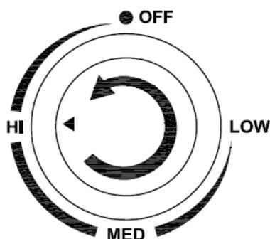
6. If ignition does NOT occur in 5 seconds, turn the burner control knob off, wait for 5 minutes to allow gas to dissipate. Repeat the lighting procedure.
