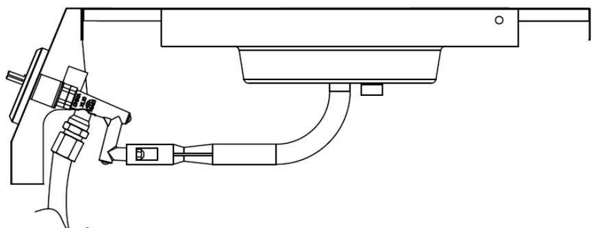
**Step 18:** Insert the connector of ignition wire to the terminal of ignition electrode of the side burner assembly as shown below.
