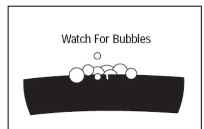
3. If a leak is present, immediately turn off the gas supply and tighten the leaky fittings.
