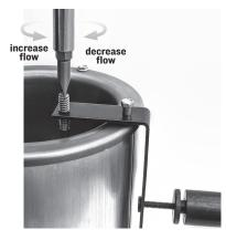
With an ingot mold placed under the pour spout, lift the pour knob and observe the flow. Rotate the valve rod clockwise to decrease flow. As the metal is consumed, you will need to rotate the valve rod counterclockwise to maintain a uniform flow. Do not rotate the valve rod too far counterclockwise as continuous flow will occur. As the valve spout ages, it may corrode or accumulate debris. Should your valve begin to drip,
