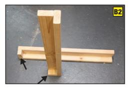
Assemble the legs as pictured above. It is a good idea to pre-drill all holes in the members that the screws go through first. Apply wood glue along all surfaces that are to make contact. Glue and screw the  $2'' \times 4''$  wood blocks at the bottom of each set as shown. Before you finalize this step please refer to B3.
