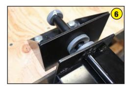
Assemble the vise half to the bracket. You will note that the clutch has fascia teeth that allow it to engage at any angle. When the knob "A" is tightened and the clutch teeth are fully engaged it will hold the vise in position.
