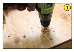
Place the vise mounting bracket on the bench top and mark the centers of the 4 mounting holes. Using the ½" drill bit drill 4 holes.
