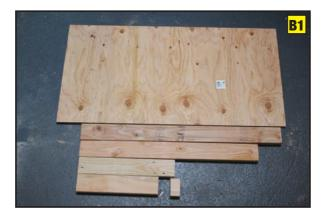
These are the materials that you will need to construct a bench that has a  $2' \times 4'$  top, with the top of the bench 36'' to 37'' above the floor.
