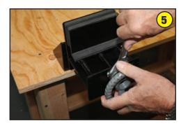
Thread the handle onto the shaft. Make sure that the #3 hex nut is in place first. Please note that the handle has a left hand thread, therefore, you will be turning it counter clockwise. Using your wrench hold the #3 nut in place and rotate the handle counter clockwise so it solidly engages against the nut and then tighten so the handle does not come loose. You will now be able to use the vise by rotating the handle.
