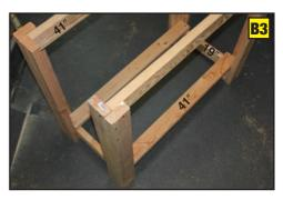
The legs are not identical within each pair one is a mirror image of the other. This is how the partially assembled bench frame will appear with the 41" and 19" 2 x 4's in place and the legs properly oriented. Glue and screw.
