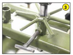
Install the T bolt. The end of the T bolt rides against the flat part of the shaft on the V notch. If you loosen the T bolt too much the shaft will rotate, if you tighten the T bolt so it's making firm contact with the flat side of the shaft and then back it off ½ of a turn you will be able to operate the capstan knob and this will move the V notch up and down. When you are at your preferred elevation tighten the T bolt and the elevation will remain fixed.
