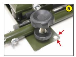
The rest and the grip arms must be securely anchored to the bench top. Any motion of the rest vis-a-vis the bench will result in loss of repeatability. If the bench is concrete or attaching the rest to the top of the bench is not allowed, then you will need to build a bench rest platform which is featured further on in this booklet. Use the holes in the brackets to secure the rest. A #14 sheet metal screw will work well.
