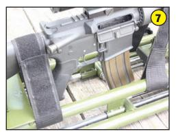
Now use the 2 Velcro straps to secure the gun. The rear strap, which will typically go around the wrist area of the stock, should be firmly and tightly secured. The forward strap is basically a safety strap and therefore, should leave about 1/4" of free play between the strap and the gun so it does not create any bedding related issues.
