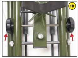
Windage can be adjusted from either side. If there is slack in the screw drive back off the hex nut retaining the knob on one side. Hold the knob on the other side then tighten the knob until contact is made. Now back off slightly and re-fix the hex nut. You may have to repeat until you get it exactly right.
