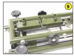
The forward gun support can be located at any of 3 locations to accommodate various gun lengths.
