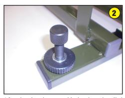
After the elevation assembly has been installed install the 4 leveling jacks by first screwing a locking collar onto the shaft and then threading the leveler onto the threaded hole.
