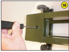
If there appears to be some slack in the windage assembly, this can be solved by tightening the Phillips screw that can be seen through the hole in the rear platform. Tighten the screw with a #2 Phillips screwdriver until it stops and then back it off 1/16 of a turn to avoid binding.
