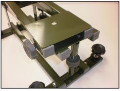
The windage is relatively straight forward. By rotating the knob you're able to move the rear of the rest either left or right and by using both the windage and elevation adjustments you're able to dial in your sight so it is dead on the point of aim.
