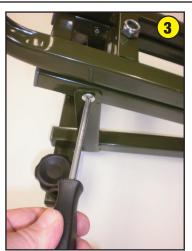
Center the upper rest assembly between the uprights in the lower assembly, align the holes as shown and attach with 1 shoulder bolt from each side. Tighten until snug, but not too tight that the rest binds.
