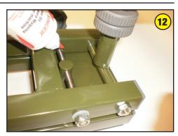
Use acid free machine oil to lubricate the threads or both the windage and elevation screws.
