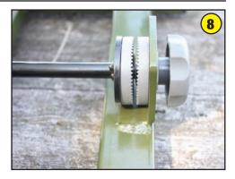
The spring helps to keep the clutch halves apart during rapid elevation. When the knob is tightened the clutch engages and holds the setting.
