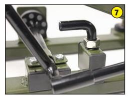
Install the elevation "memory" Stop bolt. The elevation can be set to a predetermined setting. This is simple but effective.
