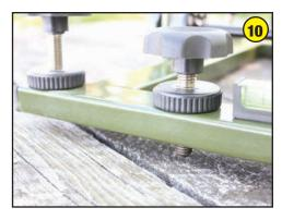
If you are on a flat bench with a smooth surface, the rest will pivot around the pivot jack. For turf or uneven surfaces use a piece of plywood or Masonite - or even stiff corrugated cardboard.
