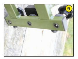
To pivot the rest, raise all four elevation jacks and lock them in place. Then lower the center pivot jack about 1/2"and lock it in place.
