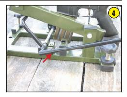
Thread the handle into the threaded socket on the end of the crankshaft. Hand tightening is sufficient.
