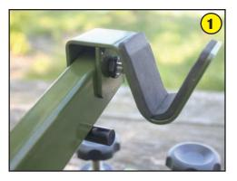
Use the M-10 shoulder bolt and hex nut to attach the forward gun support. The washer fits between the "V" notch support and the arm. If it has been factory assembled disregard this step.
