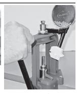
LOWER ram (raise handle) to seat the primers. The primers should be flush to slightly below flush when properly seated.
