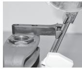
**INSTALL** correct primer feed assembly LARGE white trigger assembly SMALL black trigger assembly into primer feed bracket.
