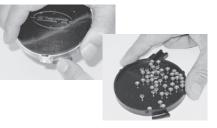
DEPRESS primer latch on tray, rotate counterclockwise and lift off cover. Place no more than 100 primers in tray; shake side to side to tip primers upright
