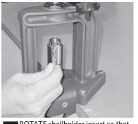
ROTATE shellholder insert so that primer arm in on right side of Classic Cast press.
