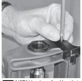
INSTALL primer feed bracket with supplied 10-24 screws. On Lee Turret Presses, use bracket provided with press (2006 and newer). Older presses can be updated with **UPDATE KIT 90042**
