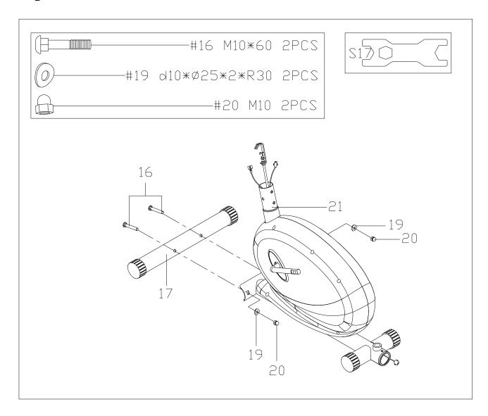
Secure Front stabilizer (17) to Main frame (21) with Bolts (16), Arc washers (19) and Nuts (20).
