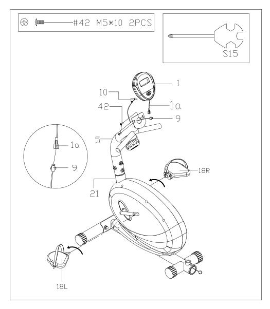
A. Connect Computer wire (1a) with Sensor wire a (9), then secure Computer (1) to Handlebar post (5) with Screws (42). Insert Sensor wire b (10) into the back of Computer (1).
