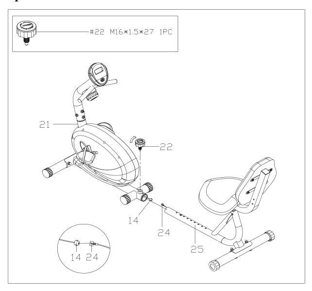
A. Connect Sensor wire d (14) with Sensor wire 5 (24), then secure the Rear main frame (25) to the Main frame (21) with the Knob (22).
