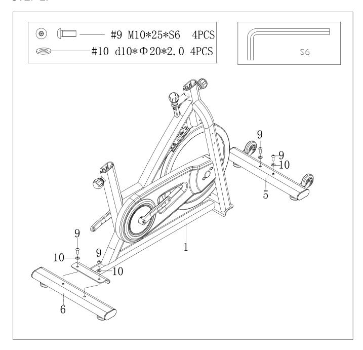
A. Secure front stabilizer (5) and rear stabilizer (6) to main frame (1) with screws (9) and washers (10).
